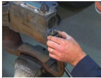
FIGURE 78 - POSITION THE NEW BUSHING
