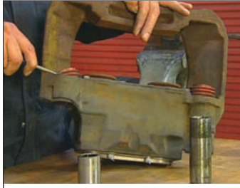
FIGURE 68 - REMOVE THE RETAINING RINGS, GUIDE PINS, AND BOOTS
