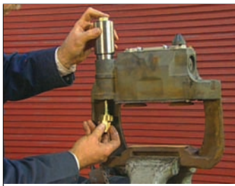
FIGURE 70 - INSTALL THE REMOVAL TOOL
