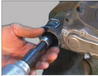
FIGURE 67 - REMOVE THE CALIPER BOLTS
