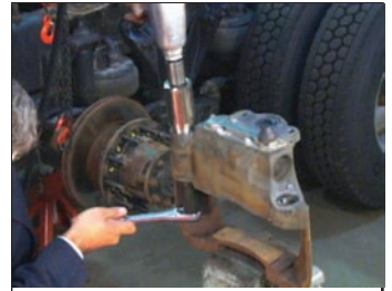
FIGURE 71 - REMOVE THE LONG GUIDE PIN
