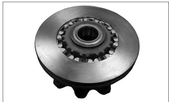
FIGURE 90 - INTERMEDIATE ELEMENTS (SPACERS) INSTALLED
